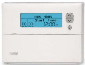
The LuxPro PSP722E meets all thermostat requirements for the V-star 3 speed plus it is a 7 day programmable thermostat. <u>This thermostat must be programmed as a heat pump t-stat to work on the Hydro-Temp system.</u> Follow the instructions in the next section for programming the t-stat for heat pump mode. The following instructions can be found in the installer manual for the LuxPro PSP722E:
