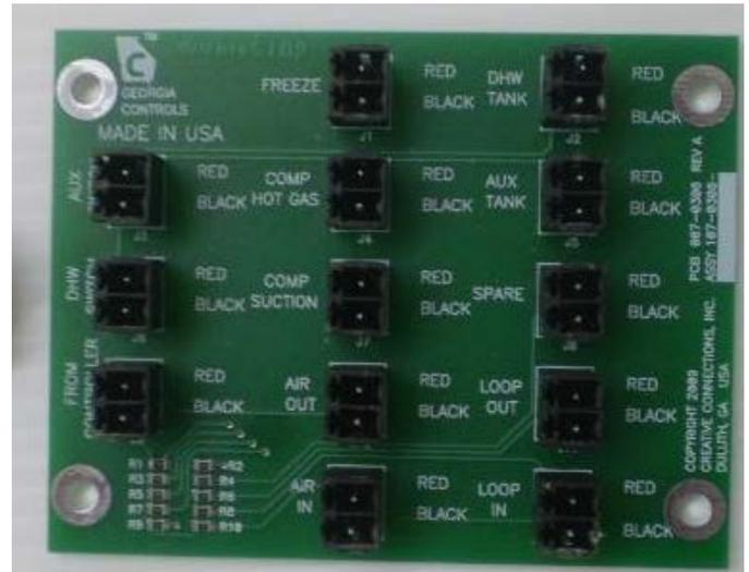
All sensors communicate through a one wire bus to the control board. Sensors are connected to the small board pictured above on the right. This board is then attached to the control board. This allows for easy sensor replacement or servicing. On/Off toggle switches are also connected to the small board to turn on and off the priority options as needed. **The polarity of all sensors must be matched Black to black and red to red.** The spare input can be used for the humidity sensor if used.
