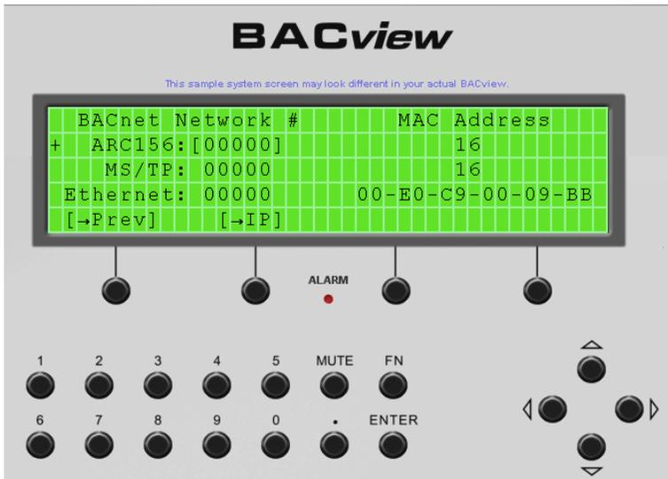
While at any of the above screens you can press and hold down the FN (Function) key plus the 9 key. This will bring up the Network screen. Press the arrow keys to scroll to Arc156. Press enter to edit the existing Arcnet network number. This number needs to be set to zero, and then press enter.
