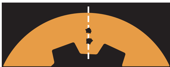
Cross-section showing portion of corrosion (leak)
