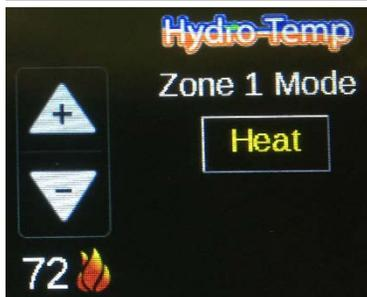
In the heat mode only the heating set-point will be displayed below the plus and minus (up and down) arrows.
