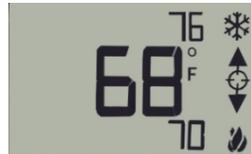
**The zone mode icon** will display as a snowflake when in cool mode and a flame when in heat mode. They will alternate when in auto mode. Changing modes will be discussed later from the Info Screen setup.
