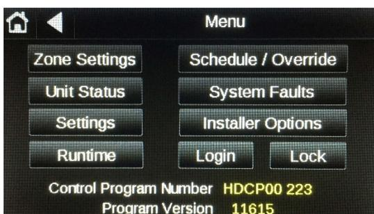
To access the Installer Options from the menu screen press the installer options button. The password required window will pop up. Press OK and enter your dealer password.
