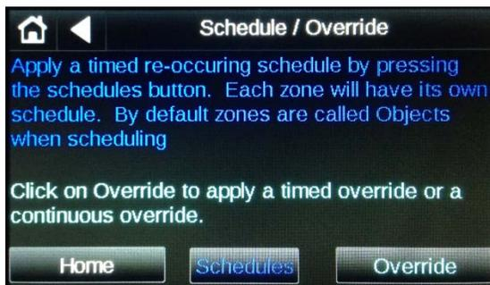
We will first discuss the override option. This is the easiest way to set the unit for an occupied mode. There are two options here. One is the continuous mode and the other is timed mode. If the “Continuous” button is selected, a pop-up will appear that provides the option for “on/off”. If “On” is selected the zone will be occupied 24/7 much like having the “Occupied Sensor” jumper in place in the electrical box.
