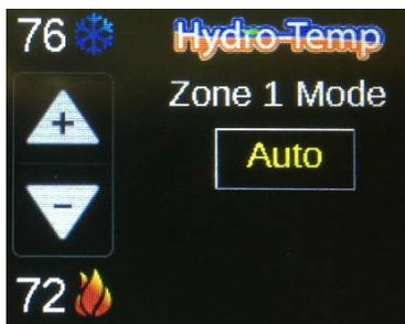
In the auto mode both the heating and cooling set-points will be displayed above and below the plus and minus (up and down) arrows.
