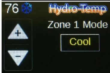
In the cool mode only the cooling set-points will be displayed above the plus and minus (up and down) arrows.
